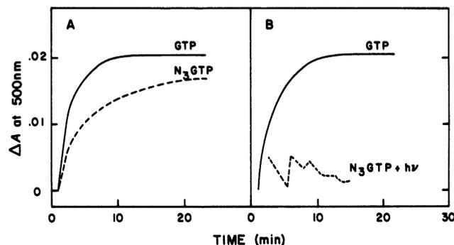
FIG. 3. Effect of photolysis of tubulin polymerization of 8-N<sub>3</sub>GTP. GTP-dependent tubulin (0.5 mg/ml) was incubated at 0° in 0.1 mM MES, pH 6.4/0.5 mM MgCl<sub>2</sub>/1 mM EGTA/1 mM GTP or 8-N<sub>3</sub>GTP for at least 30 min. (A) Polymerization was initiated by transfer to a heated (37°) cuvette chamber. Each solution was depolymerized by incubation at 4° for 1 hr followed by a 2-min photolysis in the cuvette at a distance of 1 cm. (B) Repolymerization was initiated as before.
