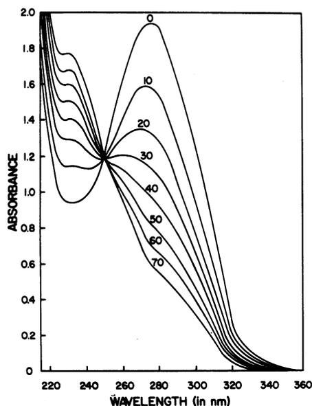
FIG. 2. Effect of photolysis on ultraviolet spectrum of 8-N<sub>3</sub>GMP. The ultraviolet profile of 8-N<sub>3</sub>GMP (0.16 mM, neutral pH) is extensively altered by exposure to ultraviolet irradiation for increasing lengths of time (10-sec increments). Photolysis was performed at a distance of 1 cm with a UVS-11 Mineralight.
