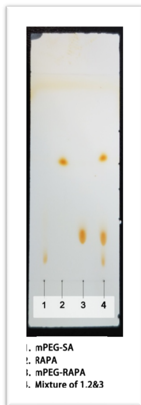
Figure S1B: TLC analysis photograph (silica gel, 10% MeOH in \text{CH}_2\text{Cl}_2 ) of the mPEG-SA (1), rapamycin (2), mPEG-rapamycin conjugate (3) and a mixture of mPEG-SA, rapamycin, and mPEG-rapamycin conjugate (4) after iodine stain. It is clear that the mPEG-rapamycin conjugate is pure, containing just a single specie.
