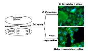
Silica sols are generated via vapor deposition of tetramethyl orthosilicate (TMOS) into an aqueous medium. Subsequent mixing, under various experimental conditions, of eukaryotic and mammalian cell types with silica sols results in encapsulation of cells in tunable silica structures (represented by green fluorescence).
