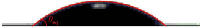
Figure S2: The circular arc fitted to the periphery of an equilibrium droplet with 1.0 cP viscosity.
