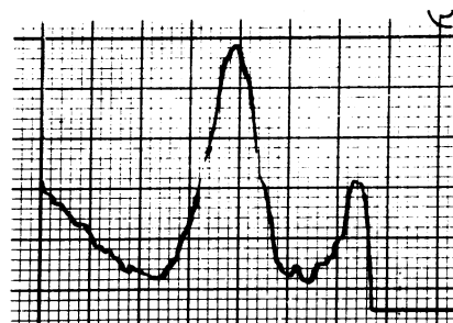
FIG. 3. Sedimentation velocity ultracentrifugation of purified mouse-liver aldolase. The enzyme was centrifuged in 2.5° double-sector cells in an An-D rotor at 60,000 rpm at 20° in 10 mM Tris·HCl-1 mM EDTA-10 mM 2-mercaptoethanol-0.1 M NaCl (pH 7.5), at a protein concentration of 0.8 mg/ml (4). The photoelectric scanner recording is the derivative of the absorbance at 280 nm.
