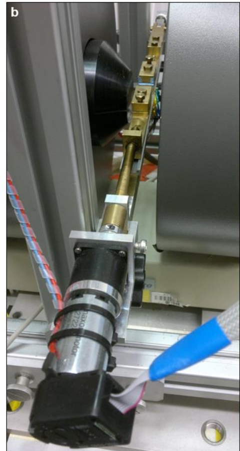
Supplementary figure 13 | The in-situ GMR stretching setup. (a) Schematic view of the setup. (b) Photograph of the motorized stretching stage between the pole shoes of the electromagnet. A close up of a contacted sample between the clamps can be found in Fig. 2b and Supplementary Movie 5.
