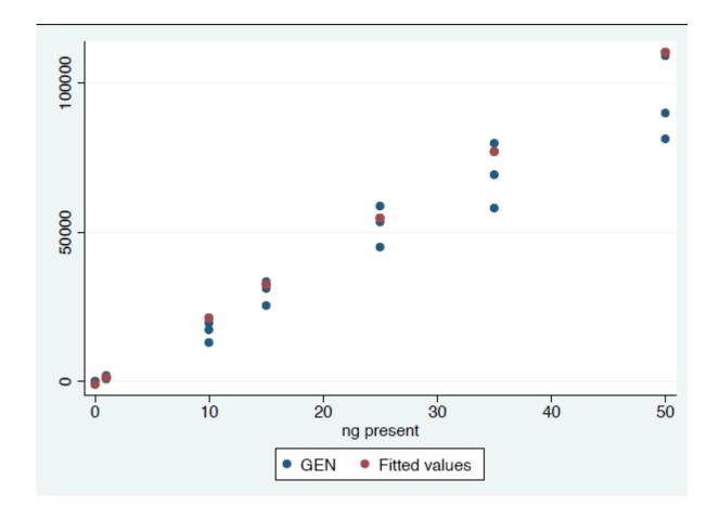
Figure S4: Genistein glucuronide calibration curve. (Y-axis: integrated area)
