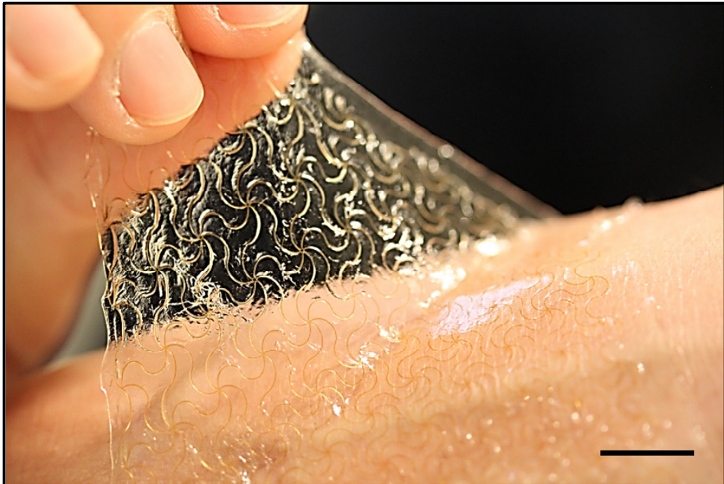
Supplementary Figure 4. Images of skin-like composite that consist of a lithographically defined PI network mesh and soft/breathable silicone elastomer sheet. The composite is softly laminated with full conformal contact to human skin and partially peeled off with stretching. All scale bars are 2 cm.
