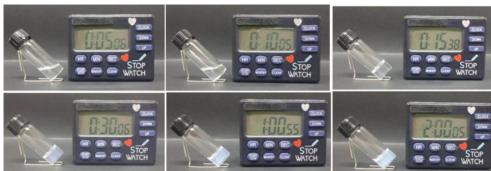
Supplementary Figure 4. The photograph for gel formation (organogel-6) of 1+2 ( 1 : 42 mM and 2 : 84 mM) in the presence of HCl (5 nmol) by increasing hydrazone reaction times.
