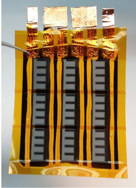
Figure S6: The finished array of 9 asymmetric cells connected 3 in series X 3 in parallel.
