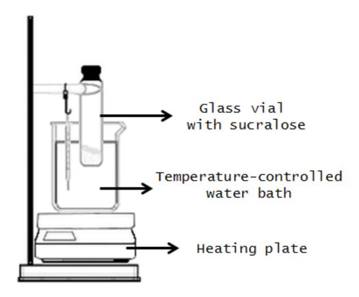
**Supplementary Figure 1 (Figure S1).** Schematic representation of the experimental setup for the thermal evaluation of sucralose, prior to HRMS analysis.
