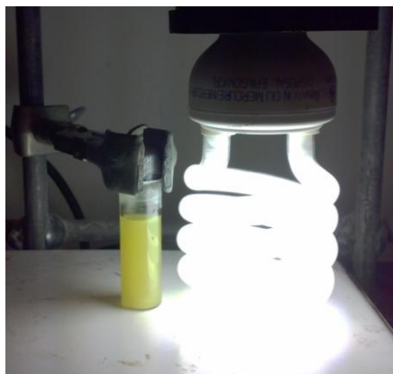
Fig S6: Photoredox cross-coupling reaction set-up (0.5 mmol scale)
