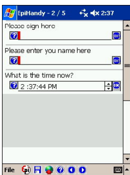
Figure 6d. Time: The time-function is mainly to record the actual time at the interview situation. If the question asks you to record another time, it can be entered by activating the automatic time and adjusting it.
