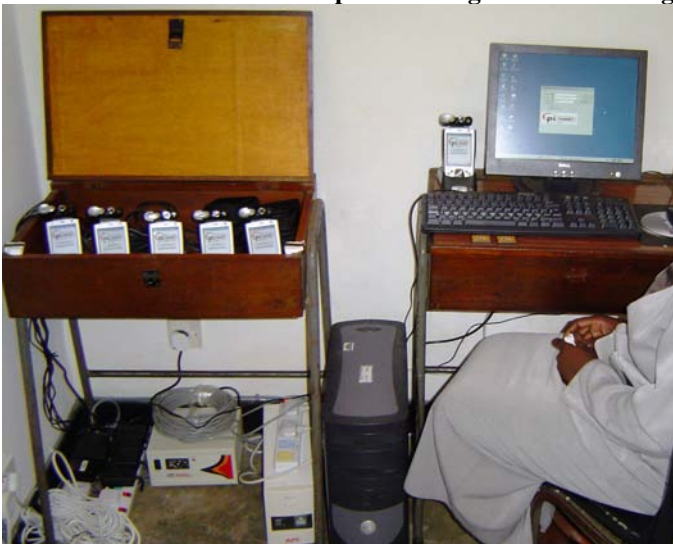
Figure 10. Initial setup of the EpiHandy server in the office where synchronisation with the handhelds takes place.
