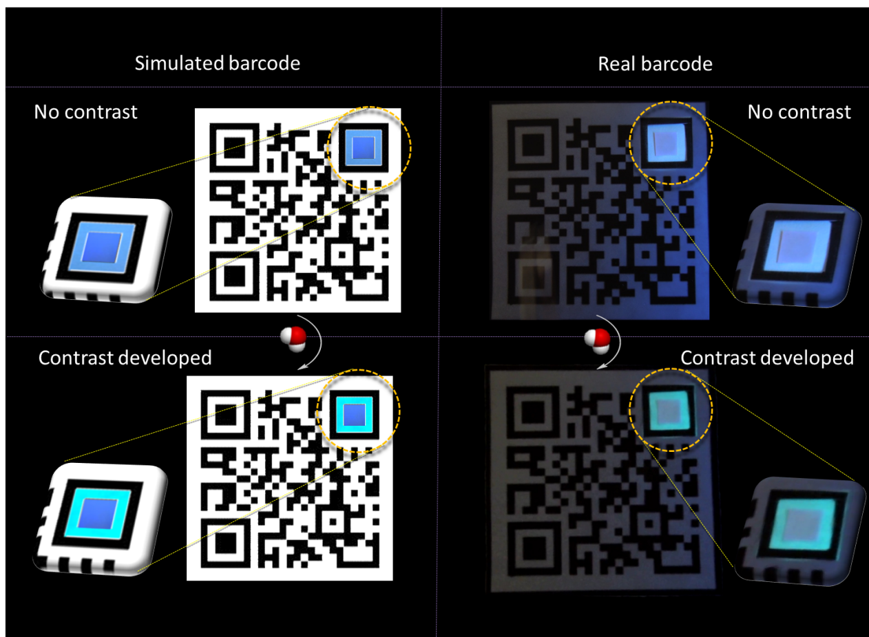
Supplementary Figure S21 | Printed barcode. Barcodes were printed with ordinary ink and the defect sites were filled with PE1 and PE3 coated films. Similar optical contrast was developed in the real experimental barcode as observed in the simulated barcode.
