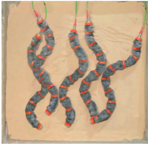
Movie S4. The snake robot performing reversal turning in a sand bed due to a 180^\circ phase shift in the vertical wave.
