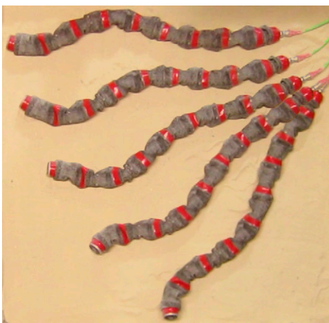
Movie S3. The snake robot performing differential turning in a sand bed due to an amplitude gradient in the horizontal wave.
