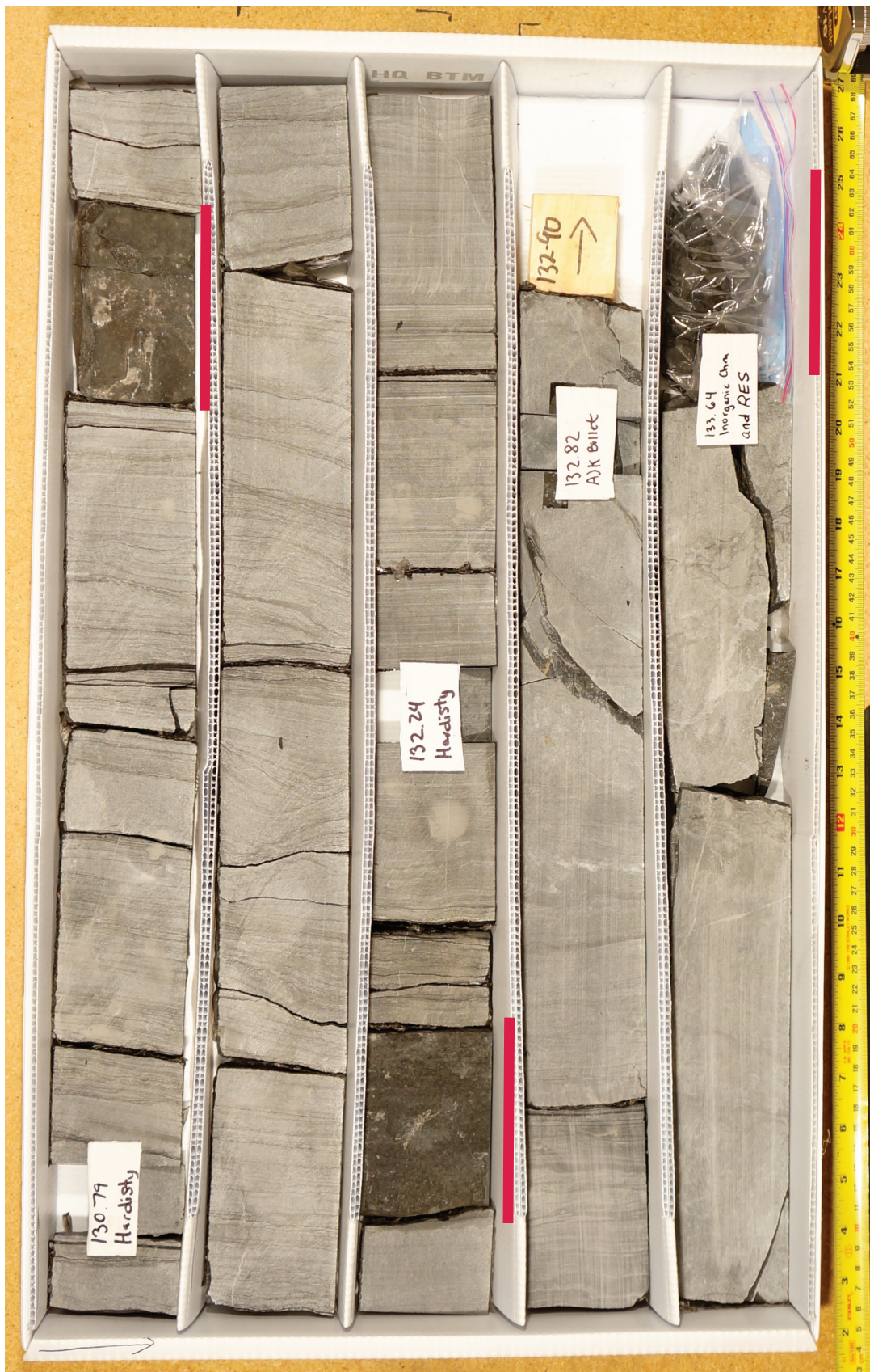
Figure S3. Photograph of Stylocumulates in the upper Carawine Dolomite of AIDP 2. The samples photographed in the core tray are from 130.75-133.67 m. Red bars to the right of the core mark examples of the dark, cm-scale stylocumulates within the surrounding dolarenite. Photograph courtesy of Moutusi Roy (ASU).
