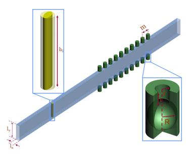
S.4. Geometric parameters of the unidirectional system.
