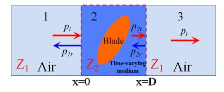
**S.2. Schematic of a waveguide section with three regions.** Medium in region 1 and region 3 is air while region 2 contains the time-varying medium. Here, the length D of the effective medium region is 0.02m in both simulation and experiment. The blade is placed in the center of this region.
