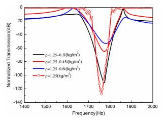
**S.8. Normalized transmission curves for the band-stop filters considering air loss via full** wave simulations. Air loss can not be ignored in experiments. We defined the mass density in resonance cavity as  $1.25kg/m^3$ ,  $(1.25-0.3i)kg/m^3$ ,  $(1.25-0.45i)kg/m^3$  and  $(1.25-0.6i)kg/m^3$ , respectively. The results can give an explanation for the differences in filters' performance between simulations and experiments.
