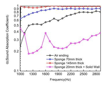
**S.5.** Acoustic absorption coefficient for various termination conditions. Since 145-mm-thick sponge has the best absorption performance among these four termination conditions, it was used exclusively in our experimental investigation to seal the waveguide.
