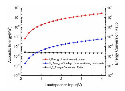
S.6. Experimental results for acoustic transmission and energy conversion ratio through the elliptical blade as a function of loudspeaker input voltage.  $I_0$  is the input energy of the input acoustic wave and  $\sum I_n$  are the sum of the output energy of all the high order scattering components generated via time-varying acoustic scattering. Energy conversion ratio here is defines as  $\sum I_n / I_0$ . From the data shown in this figure, the time-varying acoustic scattering we
