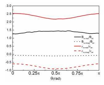
**S.3. Experimentally deduced effective parameters.** The time-varying medium in our system is anisotropic and thus tensors should be used in perturbation theory.  $B_{xx-real}$  ( $\rho_{xx-real}$ ) and  $B_{xx-imag}$  ( $\rho_{xx-imag}$ ) correspond to real and imaginary part of effective modulus (effective density) tensor element responsible for the collinear scattering process along x-axis studied in this work.  $B_{air}$  and  $\rho_{air}$  are the modulus and density of air respectively.
