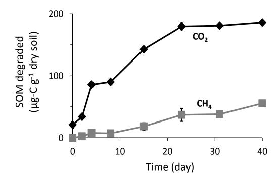
**Figure S2.** Cumulative gas production (carbon dioxide  $(CO_2)$  and methane  $(CH_4)$ ) during a simulated 40-day warming incubation experiment with an Arctic mineral soil obtained from Barrow, Alaska, USA.
