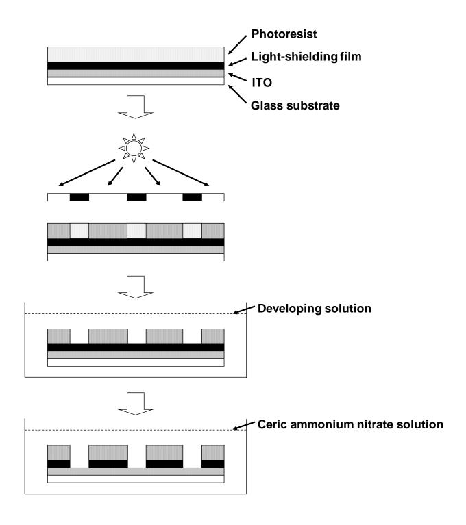
S1 Fig. Schematic Diagram of the Photolithographic Method, with Corresponding Etching, to Fabricate the Microwell Array Substrate.
