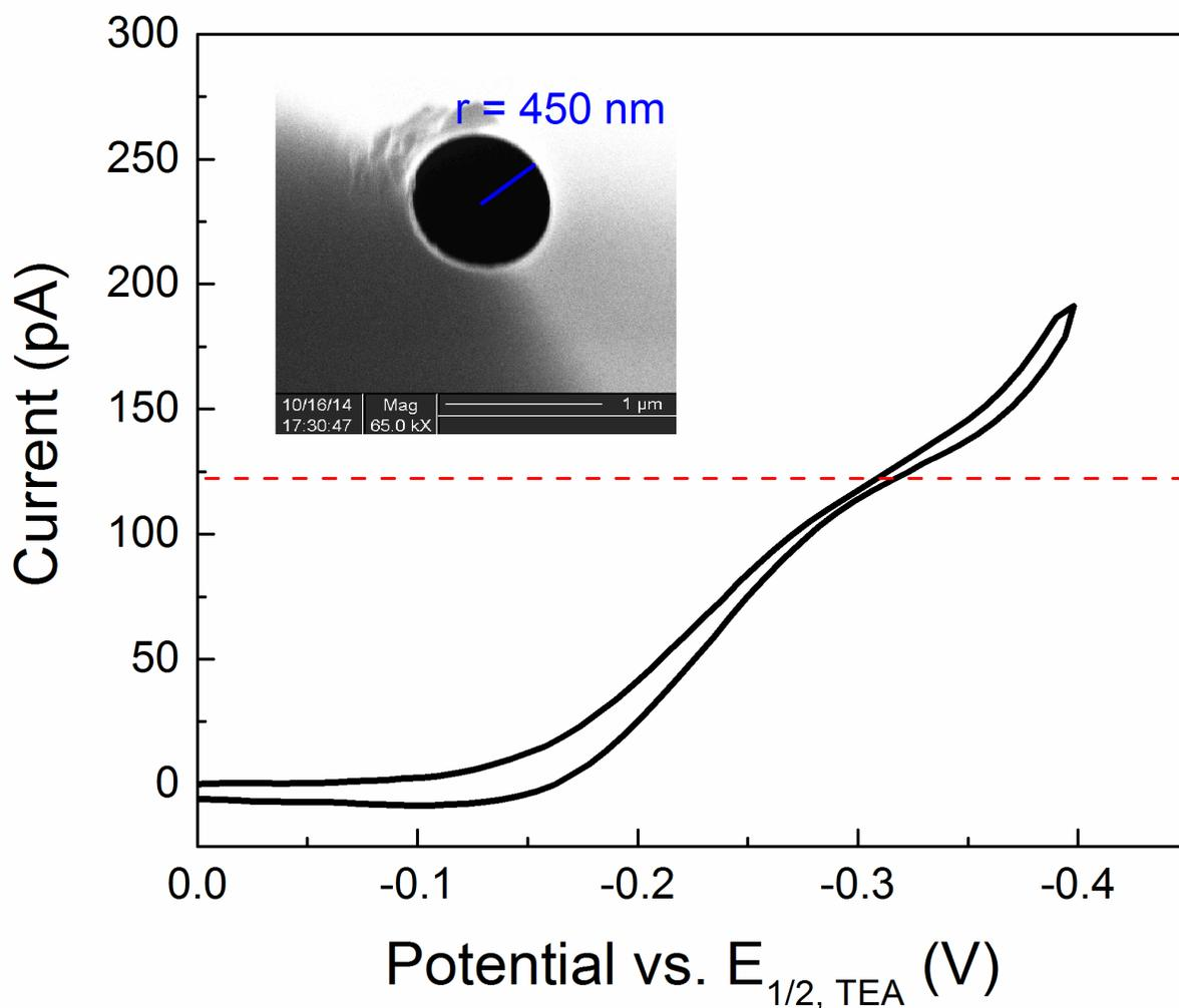
**Figure S2.** SEM and cyclic voltammogram for one of the pipets used for calculating the diffusion coefficient of tryptamine (T) in artificial sea water (ASW) via Cell 1. Concentration of T = 1 mM; Steady state current = 126 pA (red dashed line); the process shown at more negative potentials is due to the transfer of ASW. Inset: SEM image of pipet used, showing a radius of 450 nm. Calculated  $D_T = 5.90 \times 10^{-6} \text{ cm}^2/\text{s}$ .
