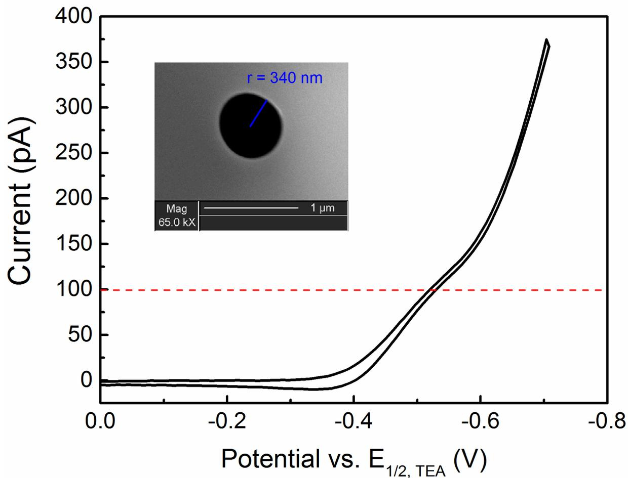
**Figure S3.** SEM and cyclic voltammogram for one of the pipets used for calculating the diffusion coefficient of serotonin (5-HT) in 10 mM LiCl via Cell 2. Concentration of 5-HT = 1 mM; Steady state current = 100 pA (red dashed line); the process shown at more negative potentials is due to the transfer of LiCl. Inset: SEM image of pipet used, showing a radius of 340 nm. Calculated  $D_{5\text{-HT}} = 6.20 \times 10^{-6} \text{ cm}^2/\text{s}$ .
