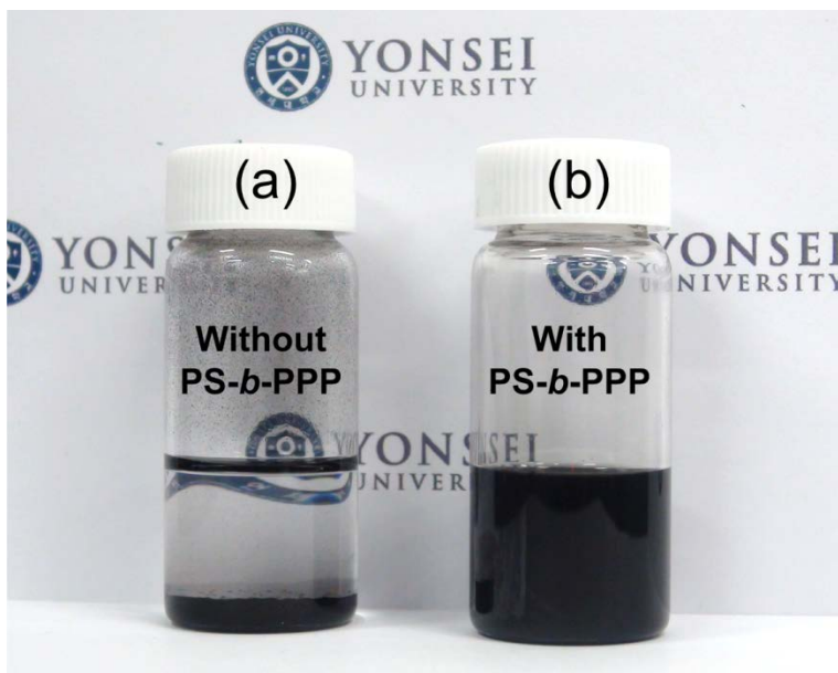
Figure S1 Photograph of 0.1 mg/mL of SWNT dispersion toluene solutions. SWNT dispersion solutions (a) without and (b) with PS- b -PPP dispersant
