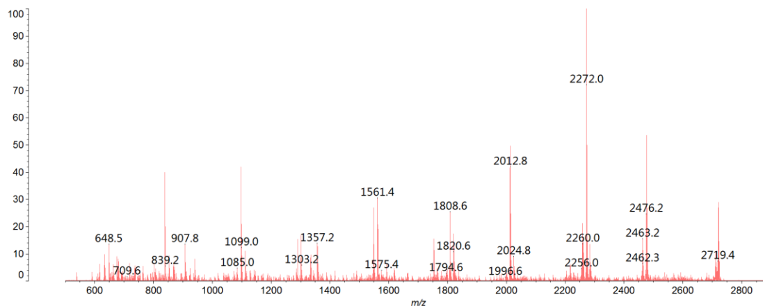
Figure S34, MALDI-TOF/TOF fragment ion spectra of the parent ions at m/z 2734
