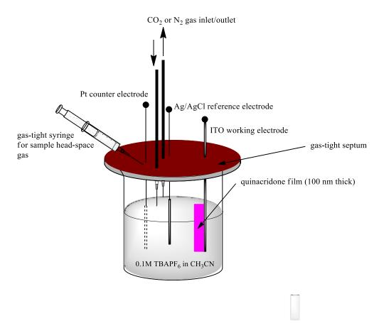
Figure S1. Electrochemical gas-tight cell used for all experiments
