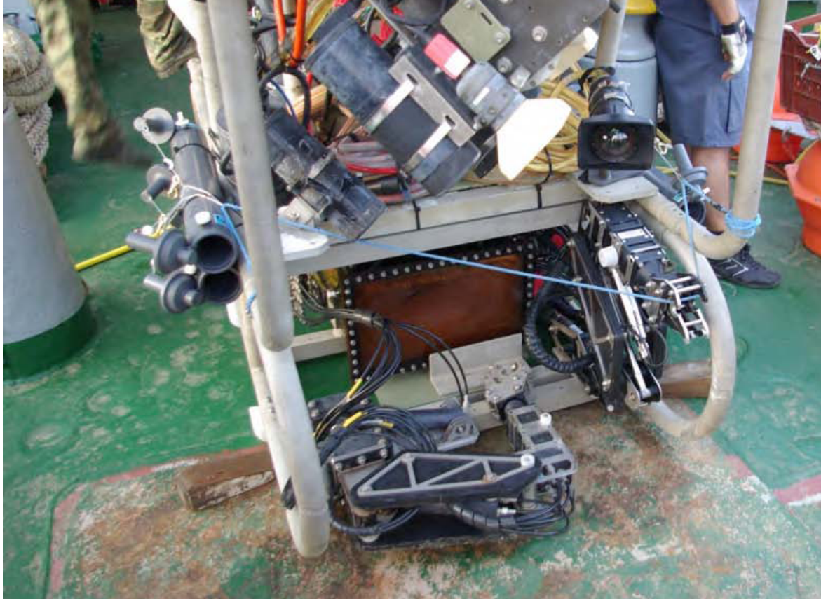
Figure S2 | Photo of the MaxRover ROV showing horizontally-mounted Niskin bottles attached to the port and starboard sides of the vehicle chassis approximately 0.5 meters above its bottom skids.
