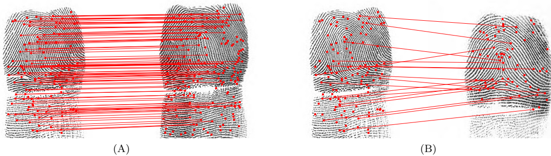
Figure S1: Fingerprint comparison using minutiae configuration. Minutiae correspondences are shown for (A) a genuine fingerprint pair and (B) an impostor fingerprint pair. The fingerprint match (similarity) scores obtained by the COTS-2 matcher are (A) 389 and (B) 11 (note that the match score corresponding to false acceptance rate (FAR) of 0.01% is 24).
