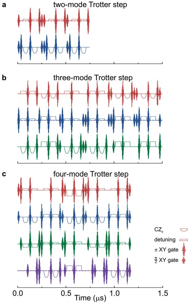
**Supplementary Fig. 1. Pulse sequences.** (a) Two-mode Trotter step. (b) Three-mode Trotter step. (c) Four-mode Trotter step. Shown are entangling gates as well as single-qubit microwave, idle and detuning gates. The legend is in the bottom right. XY pulses are 25 ns long.
