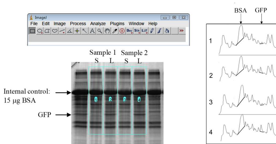
Figure S2. Quantification of the soluble fraction of GFP UV in whole cell lysis using Image J. Bovine serum albumin (BSA, 15 μg) is used as an internal control. S: supernant; L: crude cell lysis.
