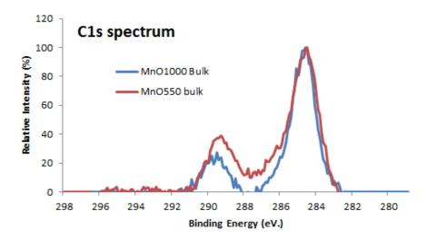
**Supplementary Figure 1:** Normalised and mean (n=3) XPS scans of the high resolution C1s spectra for thermally treated (1000°C for 8 hours) bulk birnessite coating MnO1000 and normalised and mean (n=9) XPS scans of the high resolution C1s spectra for thermally treated (550°C for 8 hours) bulk birnessite coating MnO550
