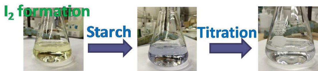
Supplementary Fig. 7 | Color changes during iodometric titration.
