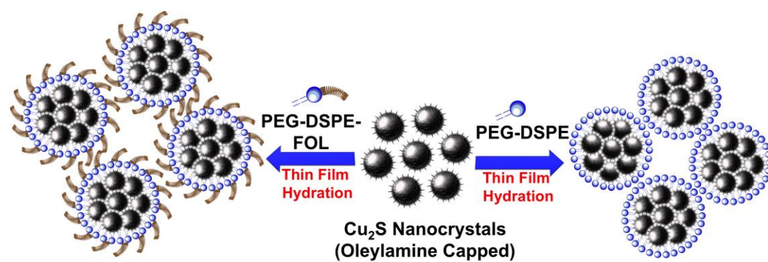
Scheme S1: Preparation of PEG-Cu 2 S and PEG-Cu 2 S-Fol NCs by thin-film hydration method.
