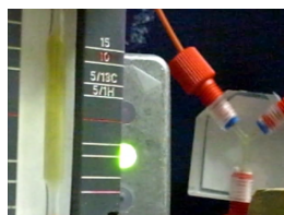
Figure S3: Distinct color change of bromophenol due to a pH change upon mixing, used to determine the timing for injection of the non-hyperpolarized sample in loop L2.
