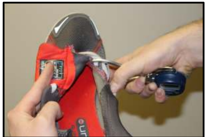
Fig C-2. The caliper must be placed at the middle of the shoe when looking from the top
