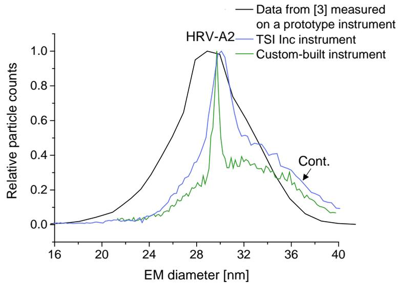
Figure S-1: Comparison of GEMMA signals obtained for a sample of native HRV-A2 on instruments of various generations. It is of note that the increasing resolution between first measurements and measurements carried out later on a conventional instrument allowed for discrimination of peaks corresponding to intact virions and a contamination of HRV-A2 preparations. The resolution (in terms of peak broadness) is substantially improved on a custom-built instrument.
