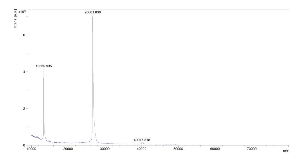
Mass spectrum of yTIM obtained in a MALDI-TOF/TOF AutoFlex Bruker instrument. 2,5 dihydroxybenzoic acid was used as matrix.
