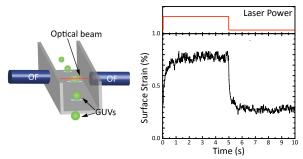
A dual-beam optical trap (DBOT, left) is used to characterize a viscoelastic stress-strain response in a lipid bilayer vesicle (right).
