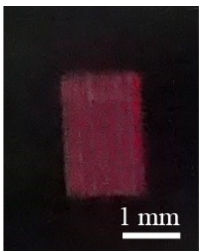
Figure S2 Purple EL emission from the fabricated microfluidic OLED device with integrated PLQ and 0.4wt% DBP-doped PLQ patterns under an applied voltage of 70V.
