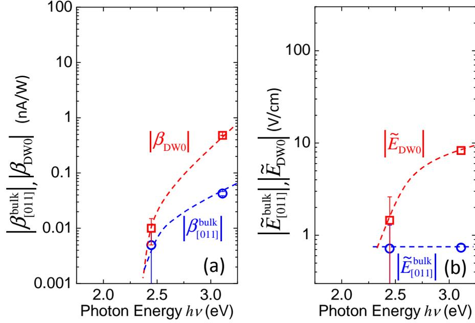
Figure S 2: Comparison of the bulk PV effect with the DW-PV effect in the BT samples: (a)  $|\beta_{[011]}^{\text{bulk}}| \equiv |\beta_{31} + \beta_{33}|/2\sqrt{2}$  and  $|\beta_{\text{DW}0}|$  and (b) the corresponding effective electric fields ( $|\tilde{E}_{[011]}^{\text{bulk}}|$  and  $|\tilde{E}_{\text{DW}0}|$ ). The broken curves are guides to the eye. The standard deviation of each data point is shown as an error bar.
