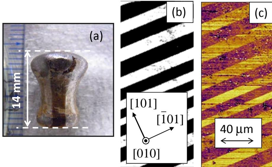
Figure S 1: (a) A Mn(0.25%)-BT crystal grown by a top-seeded solution growth method. Typical PFM images of the 90° domain structure observed in the  $\mathbf{J} // [011]$  configuration in the Mn-BT samples: (b) in-plane amplitude and (c) in-plane phase.
