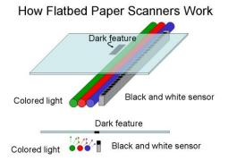
2. In order to modify this scanner for fluorescence detection, we must illuminate in the blue only (in order to excite fluorescein-like dyes) and record the light intensity in the green and red spectrum. In order to avoid collecting bright reflections in the green and
