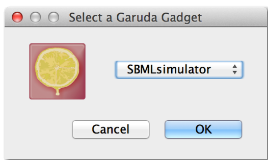
Figure 3.25: Selecting a Garuda gadget. This dialog window shows you all available Garuda gadgets that support the file type you are sending. Upon hitting the OK button, the model in the currently selected tab will be sent to the selected application.
