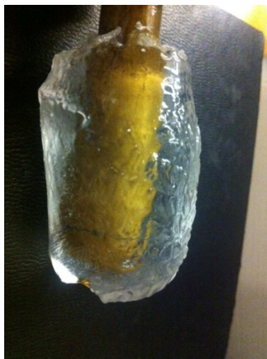
Figure S1. The polycrystalline THF crystal grown in the presence of 4 \mu\text{M} PVP.
