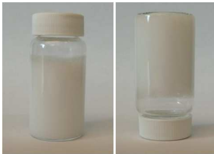
Fig. S1. Gel-like polypseudorotaxane \alpha -CD-PEG-Ts 2 inclusion complexes, in which \alpha -CDs are threaded by linear PEG-Ts 2 .
