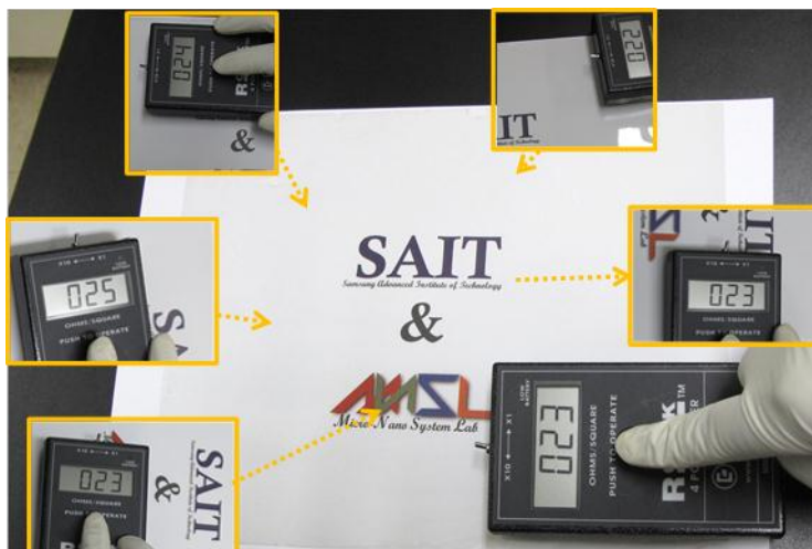
Figure S10. Visual demonstration of uniform sheet resistance of the CA-Ag NP/Ag NW TCF ( 25 \times 20 \text{ cm}^2 ) after the protective layer coating. The logos used in the figure were reproduced with permission from Samsung electronics and Sungkyunkwan University.
