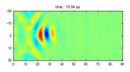
**Broadband Displacement:** Movie of the normal surface displacement measured during 50  $\mu$ s. The measured signal at each spatial position was band-pass filtered between 3.2 and 3.4 MHz and the images at each time were filtered using a square low-pass filter at a cutoff frequency of k = 0.3 mm<sup>-1</sup>.
