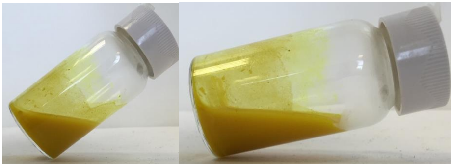
Figure S85. Photographs showing D_k after being dissolved at pH 8.5 and the pH subsequently raised to 10. Note that a gel does not form when compared to the same procedure applied to the pyridyl appended C_k .
