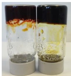
Figure S79. Gel B_e prepared by method 3 (left) and gel C_e prepared by method 2 (right) photographed 380 days after preparation at the time of writing.
