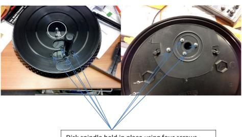
Disk spindle held in place using four screws.
