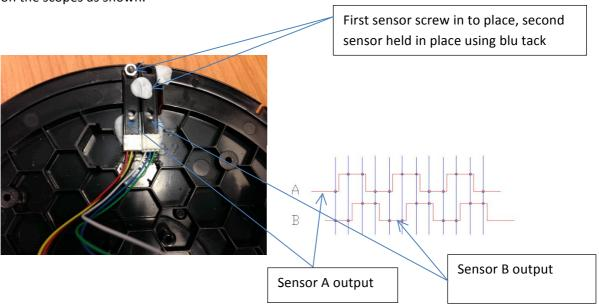
10. Now drill the second hole and screw in the sensor.
