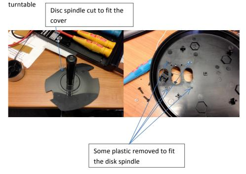
12. Drill holes and fit the disk spindle in place using four screws.
