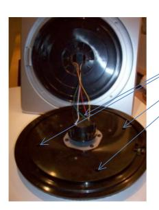
Remove 4 screws to remove cover
