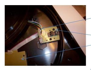
Cut the wires as close to the circuit as possible
