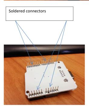
16. Build a board to connect the cable from the sensors to the micro controller
