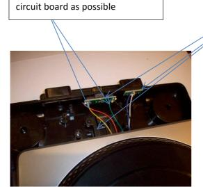
Remove the locking mechanism, connector and the reset switch
