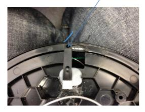
Connect the wires to the connectors. Red and white - positive 5, yellow and blue - signal, black and green - ground
