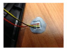
9. Place the second sensor in place using blu tack such that the output from the sensors is seen on the scopes as shown.
