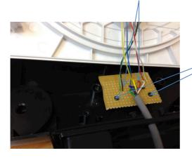
Screws to hold the vero board to the base plate
