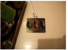
7. To fix the new sensors remove the plastic bits that are in the way and enlarge the groove that holds sensors.
