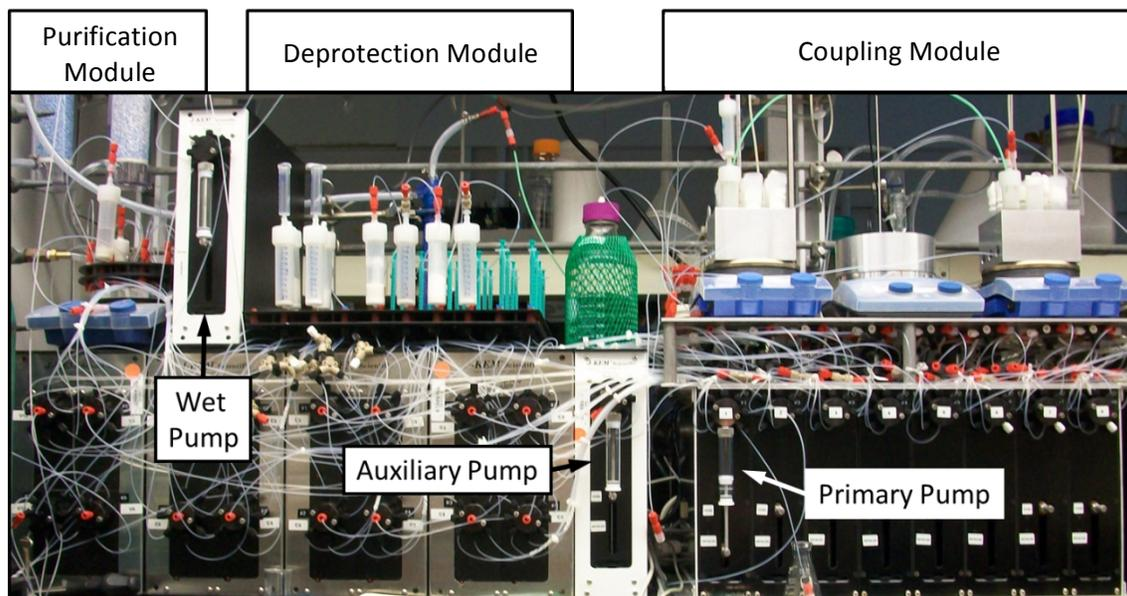
**Figure S1.** Photograph of the small molecule synthesizer.
