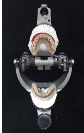
Test n° 9. Master cast assembly on a semi-adjustable articulator for fixed screw-retained restorations (TMJ movements simulation)
