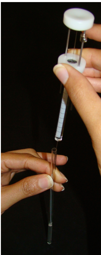
Figure S1: Titration of NMR sample with a 0.5–0.4 \mu\text{l} aliquot of NaOH using a 5.0 \mu\text{l} positive displacement syringe extended with polyethylene tubing.
