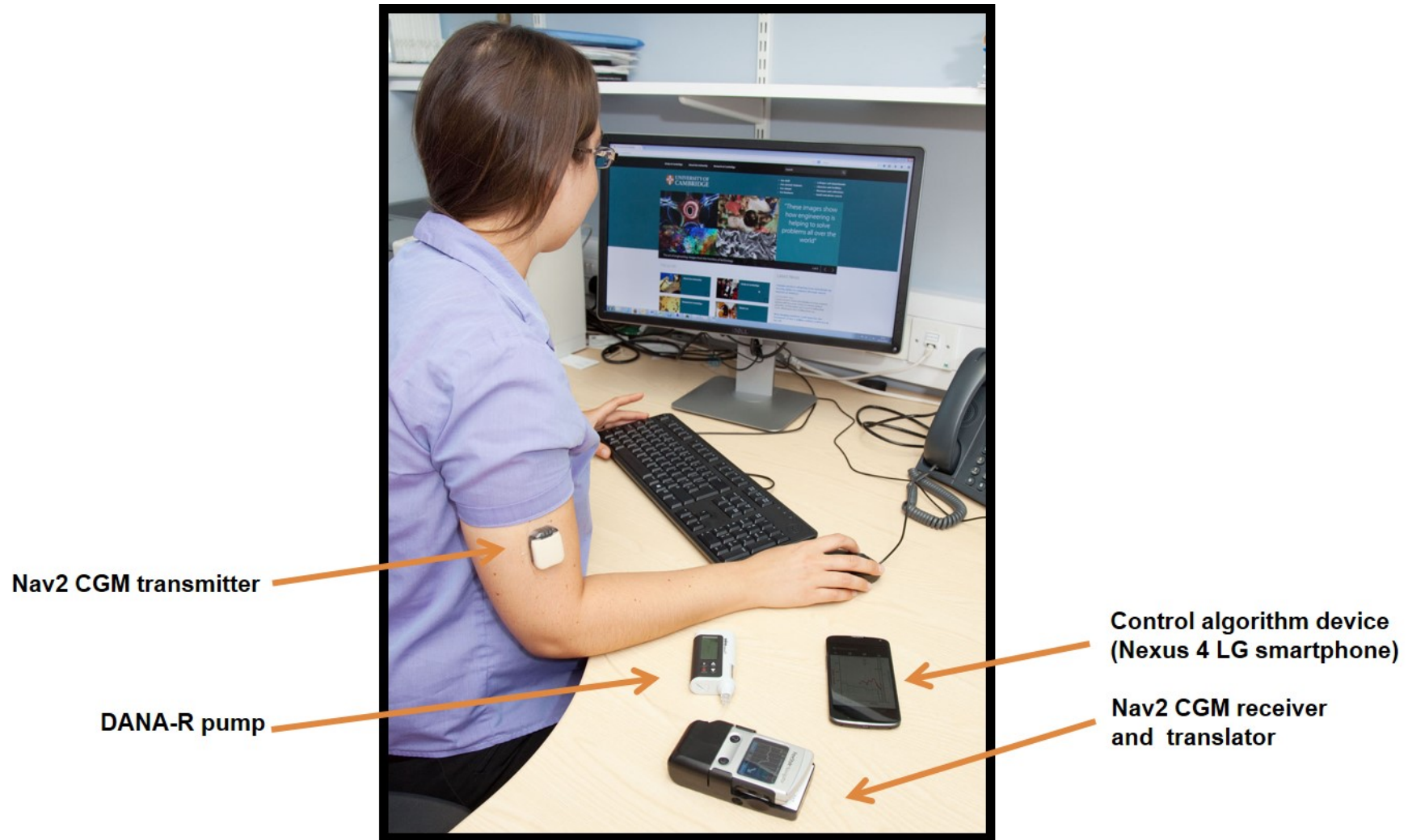
Figure S2. FlorenceD2A automated wireless closed-loop system used in the adult day-and-night closed-loop study.
