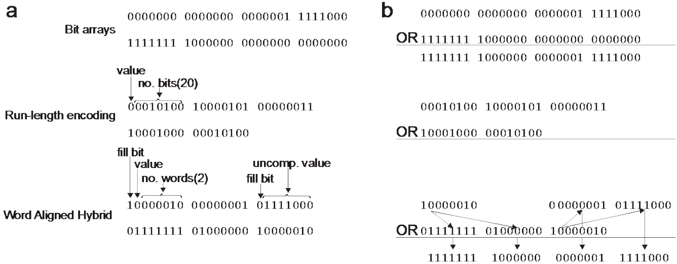
Supplementary Figure 4. A comparison of binary encodings and associated bit-wise logical operations. (a) Two bit arrays are given in three different binary encodings: the uncompressed bit array (in 7 bit words) on top, followed by the run-length encoding (RLE) and word-aligned hybrid encoding (WAH), which each add an additional bit as part of the encoding to make 8 bit words. RLE maps each set of consecutive bits to a new value that uses one bit for the run value, and the remaining bits for the number of bits in the run. WAH maps bits to one of two types of values: those that include runs and those that encode the raw binary. The first bit in a WAH value indicates if the value encodes a run (the fill bit). If that bit is set then the second bit gives the run value and the remaining bits give the run length in number of words (i.e., not number of bits as in RLE). If the fill bit is not set then the remaining bits are the uncompressed binary values. (b) The logical OR for the three encodings is given. For the uncompressed binary, the OR follows bit for bit across both values. For RLE, the logical OR is undefined (without inflation) because the two encoded values are no longer aligned and have different lengths. For WAH, the values are aligned based on their run length, then the logical OR is performed (in this case) between the value bit and the associated uncompressed values.
